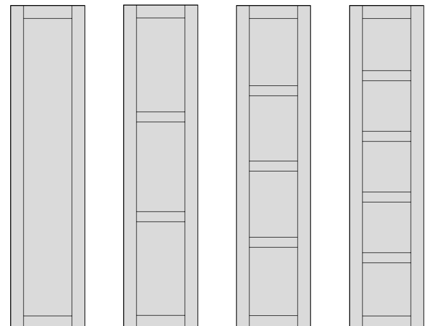
Dylan Bedroom Single Panel Door No mid-rails included* Dylan Bedroom 3 Panel Door Includes 3 separate mid-rail pieces* Dylan Bedroom 4 Panel Door Includes 3 separate mid-rail pieces* Dylan Bedroom 5 Panel Door Includes 4 separate mid-rail pieces*
